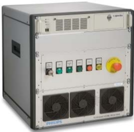
Figure 6: Electronic driver system for the high power VCSEL system.
