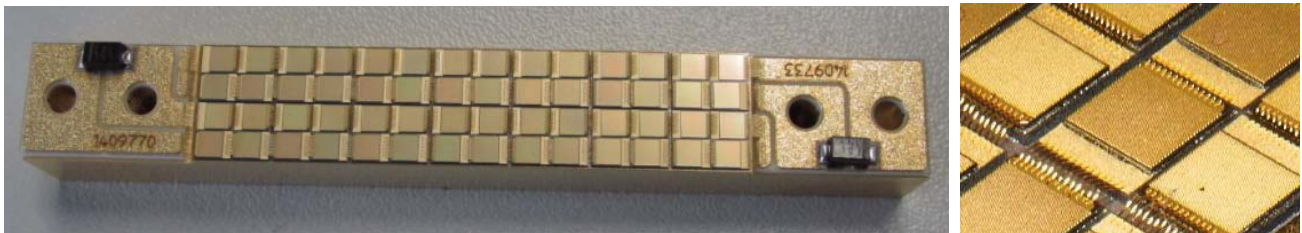
Figure 3: Assembled emitter (left) and detail of the individual chips (right).
